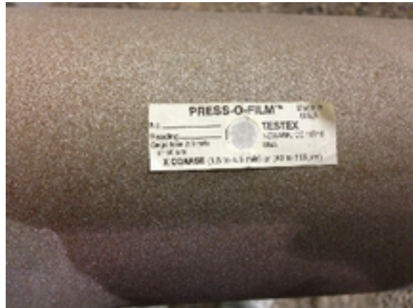
Tested tape for blast spec
